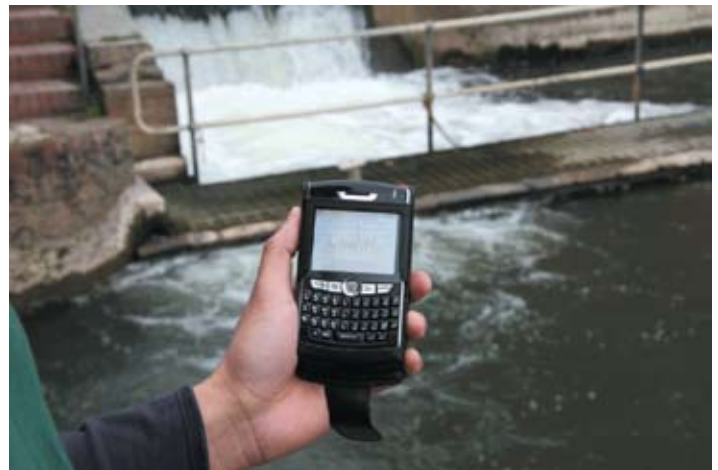
Readings every 15 minutes from automatic water quality monitoring stations. Sudden spikes in data alert managers to the first signs of CSOs or other forms of pollution entering the Thames.
