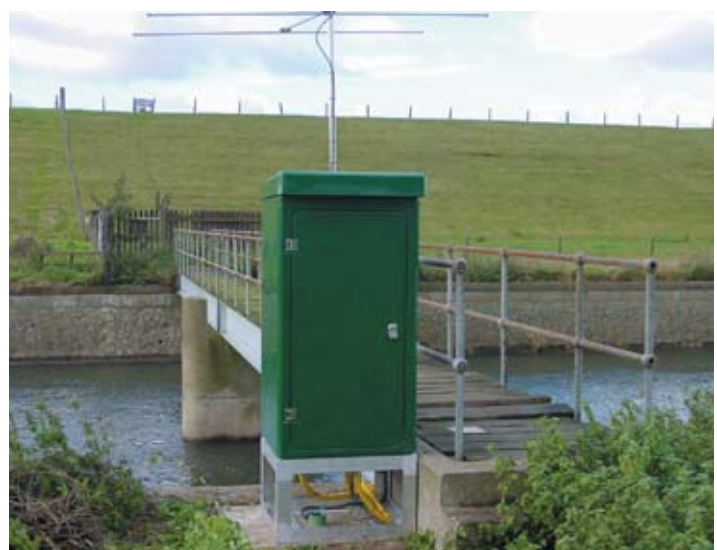
A "green box" automatic water quality monitoring station quickly provides localized data at many points throughout the Thames River
